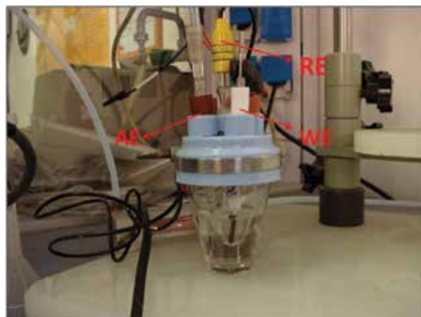
Figure 45.2. Traditional three electrode configurations: 1. RE-Reference Saturated Calomel Electrode (SCE), 2. WE-Working Electrode and 3. AE Auxiliary Platinum Electrode (by the authors, 2011).
